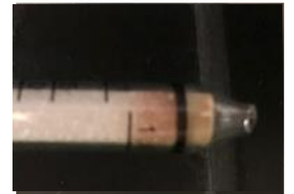
Figure 3 Detection of hydrogen peroxide release at the output of the Oxyion Series 4000. The brown color indicates that hydrogen peroxide is released at a concentration of 0.1 ppm.
