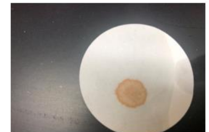
Figure 5: Addition of a 1 ul drop of 8 mM hydrogen peroxide to the filter paper shown in figure 4 shows the reddish color resulting from the: oxidation of guaiacol by hydrogen peroxide.
